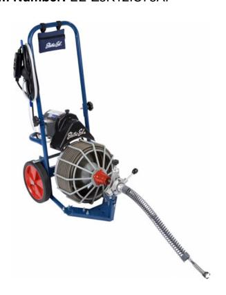
The Z5 cleans 1-1/4" - 3" diameter lines up to 75 ft. and fills the gap for those jobs that require a longer run in smaller drain lines. The auto-feed function allows the operator to advance and retrieve the cable with the push of a lever. The cable runs through a guide spring which keeps hands off the rotating cable for added safety.
