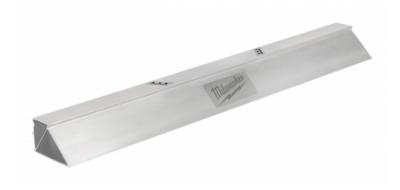
Our Screed Bars have an extra-rigid, double triangle design to transmit consistent vibrations across the length of the bar, with minimal variability. These MILWAUKEE® screed bars are constructed from lightweight magnesium to reduce the weight of the screed when in operation. The concrete power screed bar utilizes a clamp design with no holes or hardware through the bar, allowing you to quickly attach the bar at any point on the machine.
