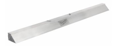
Our Screed Bars have an extra-rigid, double triangle design to transmit consistent vibrations across the length of the bar, with minimal variability. These MILWAUKEE® screed bars are constructed from lightweight magnesium to reduce the weight of the screed when in operation. The concrete power screed bar utilizes a clamp design with no holes or hardware through the bar, allowing you to quickly attach the bar at any point on the machine.
