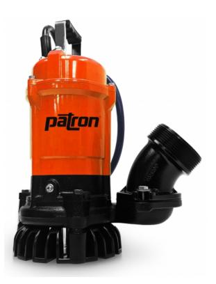
The Patron SP-35 submersible sand trash pump, with a 1 hp motor and 3-inch discharge, is a robust solution for efficiently transferring water with sand and debris. Its agitator ensures effective handling of solids, making it ideal for dewatering tasks in construction and excavation projects. With reliable performance and durability, the SP-35 pump is well-suited for handling challenging water conditions in various environments.
