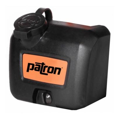
This water tank is designed to be used with Patron FP60 plate compactors. When compacting hot asphalt, a constant supply of cool water is needed on the surface to avoid hot asphalt sticking to the cold plate of the compactor. Water tanks are also ideal for very dusty applications.
