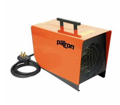
The Patron E9 is a top seller which exceeds expectations on a regular basis. It can be used in the most demanding of environments and has proven its abilities in hundreds of applications. The E9 is a 240V unit and pulls 25-37.5 amps. This means it will run flawlessly off a household stove receptacle. Make sure your receptacle is a NEMA 14-50P configuration, to ensure compatibility with our plug. The E9 produces a ton of heat, and disperses it in large areas with its 350 CFM fan.
