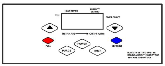
**POWER Power Button:** When the machine is in the standby mode, the display screen will be displayed in low light LED. To start the dehumidifier, press the power button. Concurrently, the display screen will light up and the unit will run in Auto mode, the default humidity setting is 10%RH, and the machine will start if the ambient humidity is above the setting.
