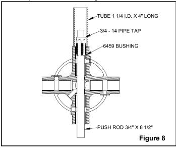
5. Use #07279 tool to ensure proper depth of bushings as shown.
